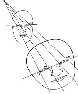
Figure 4: Cross ratio for the eye corner points
