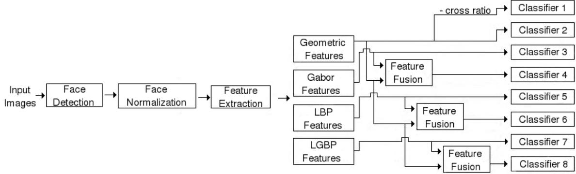
Figure 2: The overall diagram of the proposed age classification system
